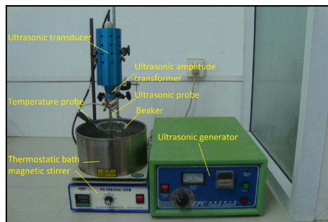
Fig. 2. The ultrasonically enhanced leaching experiment device.
